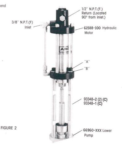
MAX. WORKING PRESSURE 360 P.S.L (25 BAR) @ 1200 P.S.L INLET.
